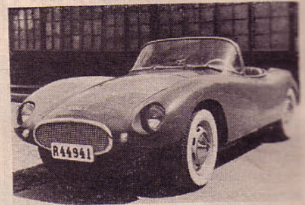
Smart styling highlights this fiberglass body shell that is made in Sweden. Called the Carina, the shell fits most cars. In this case, an A.U. 1000 (DKW) is all dressed up with the new body. Price of the shell runs just under $400.
